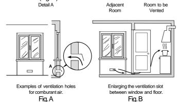
c) Intensive and prolonged use of the appliance may necessitate supplemental ventilation, e.g. opening a window or increasing the power of the air intake system (if present).
